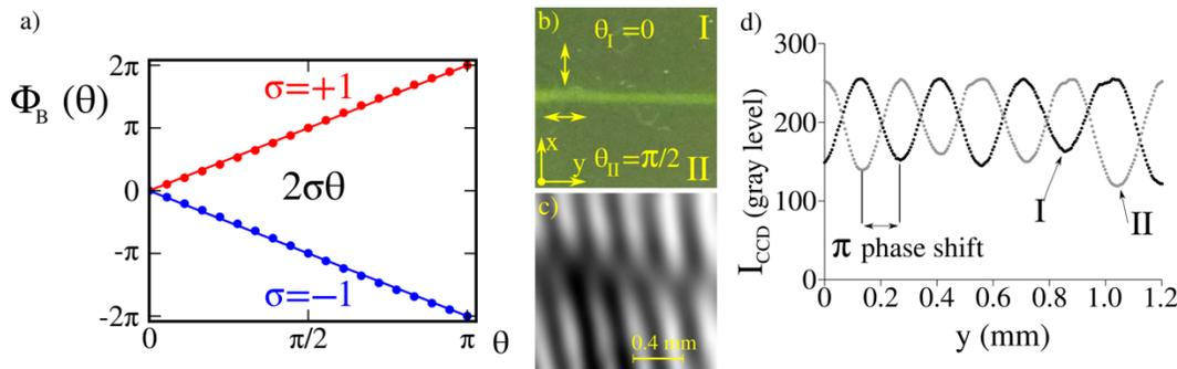
**Fig. 1** (a), Geometric phase  $\phi_B$  versus the input optical axis angle  $\theta$  of a reflected circularly polarized light with handedness  $\sigma$  (theory and simulation, resp. lines and dots). (b) Micrograph of a CLC reflector with  $\pi/2$  step-wise uniform input optical axis. (c) Plane wave interference with a reflected circular polarized beam. A  $\pi$  phase shift between the fringes in region I and II can be clearly appreciated.
