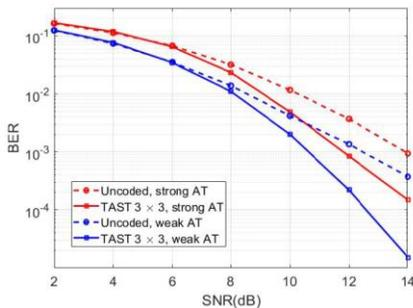
Fig.1: BER vs SNR comparison for a  $3 \times 3$  MIMO system for weak/strong AT regimes
