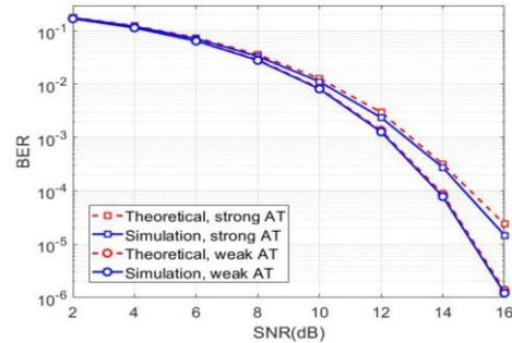
Fig.2: BER vs SNR comparison between simulations and analytical results
