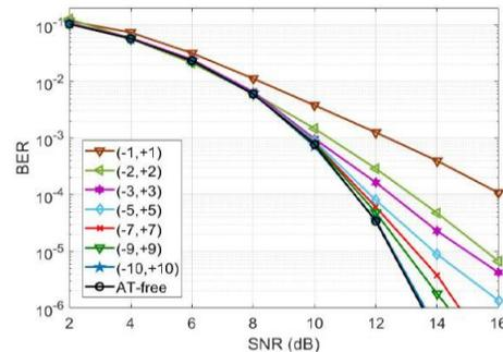
Fig.2: BER vs SNR for different sets of OAMs modes
