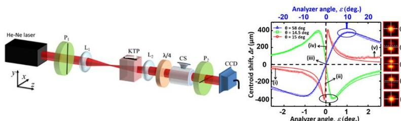
Fig. 1. (a) Schematic of the experimental setup and (b) Centroid shift as a function of analyzer angle for different orientation of the crystal.
