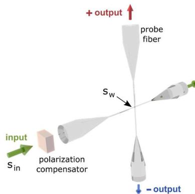
Fig. 1. Sketch of the crossed-nanofiber directional coupler. The input laser beam with the polarization state  $\mathbf{s}_{in}$  is launched into a single-mode tapered optical fiber crossed with a near-identical fiber at right angles. By adjusting the free-space compensator while monitoring the optical power exiting the ‘+’ and ‘-’ pigtails, we achieve the complete polarization control in the input nanofiber, so that  $\mathbf{s}_w = \mathbf{s}_{in}$  for an arbitrary  $\mathbf{s}_{in}$ .
