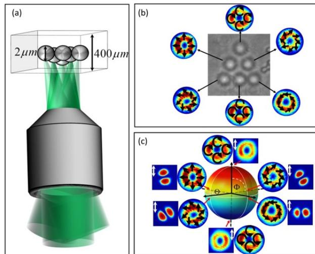
Fig. 1. An example of a vector holographic trap for the delivery of scalar and vector beams.
