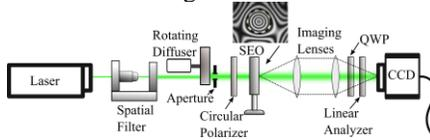
Fig. 1. Region of interest on the SEO center region is marked in dashed lines. The combination of a rotating quarter wave plate (QWP) and the linear analyzer before the camera acts as a Stokes polarimeter.
