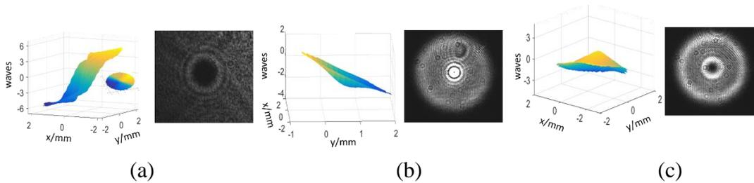
Fig. 1. Wavefront and intensity distributions that constitute of LG beams. (a) Helical, (b) incoming conical, and (c) outgoing conical.
