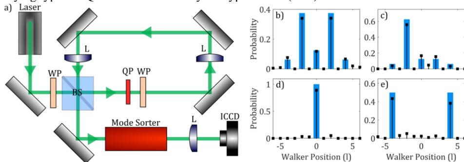
Fig. 1: a) Conceptual diagram of experimental setup. Experimental results (black) with simulated values (blue) are given for step 4 of a b) symmetrical and c) asymmetrical Hadamard QW as well as d) Not and e) Identity coin QWs.
