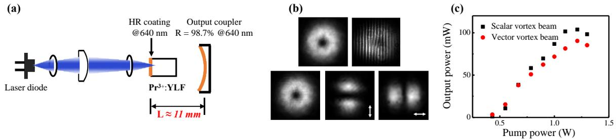
FIG 1. (a) Experimental setup for Pr<sup>3+</sup>:YLF vortex laser with the off-axis pumping. (b) Spatial form and wavefront of the generated scalar vortex output (upper row). Total intensity distribution of vector vortex beam before and after passing through a linear polarizer (arrows indicate the direction of the polarizer). (c) Power scaling of the scalar and vortex outputs.
