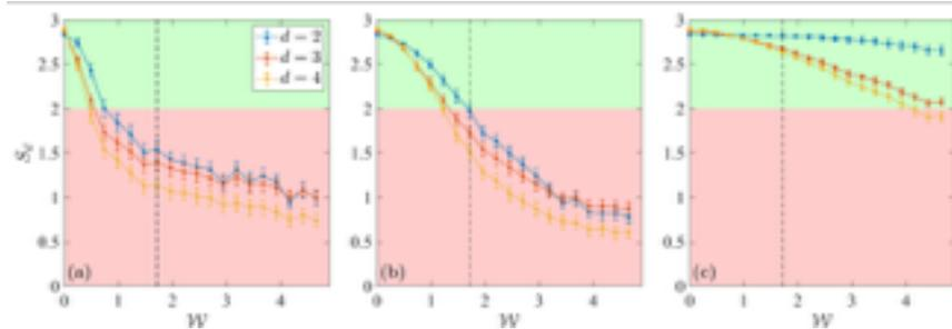
Fig.1: Bell parameters vs. turbulence strength for different degrees of AO corrections: (a) no, (b) tip-tilt and (c) ideal correction. The (red) green area indicates the region where a Bell inequality is (not) violated. The vertical line indicates the transition from weak to strong scintillation. Errors are inferred via error propagation from standard deviations around the mean of the density matrix of the output state, calculated from 500 realisations of turbulence. Figure adapted from [2].
