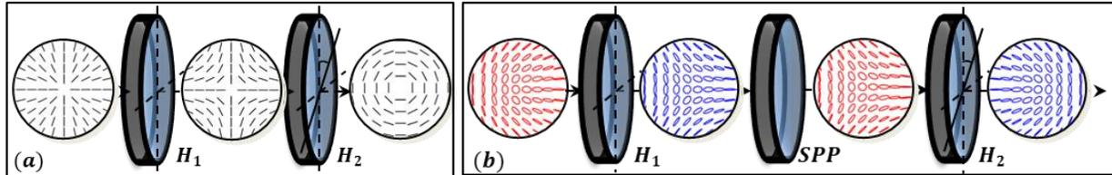
Figure 1: Orthogonal Polarization Transformation (OPT) of (a) V-points and (b) C-points. H<sub>1</sub>, H<sub>2</sub> and SPP denote two half waveplates and a spiral phase plate respectively. OPT of a V-point is two-step process, whereas for C-points, it is a three-step process.
