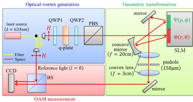
Fig. 1. Schematic of the experimental setup. BS, PBS, and QWP denote beam splitter, polarization BS, quarter waveplate, respectively.
