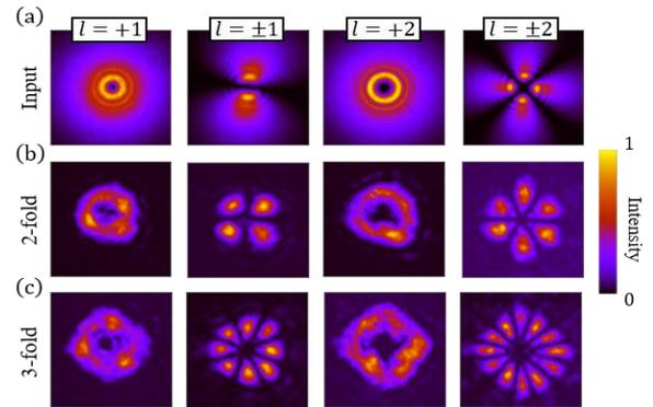
Fig. 2. Experimentally-obtained intensity distribution of (a) input, (b) 2-folded, and (c) 3-folded OAM modes by coordinate mapping.
