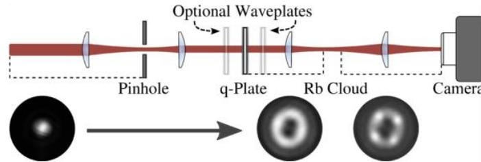
Fig. 1. Simplified account of the imaging path. The lens are selected so that both the near field and the far field of the OAM beam can be imaged on the camera. The insets are cropped images of the beam intensity, as observed on the camera under conditions of no q-plate (Left), no atomic cloud (Middle) and normal operation (Right) and serve to indicate the state of the beam at the regions indicated for  $q = 1$ .
