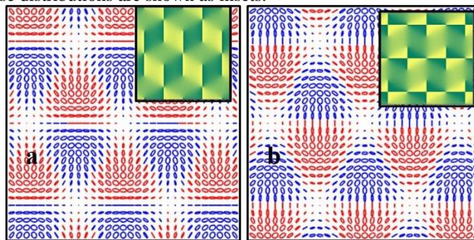
Fig. Simulated polarization distributions for three beam interference: (a) and (b) are orthogonal to each other.
