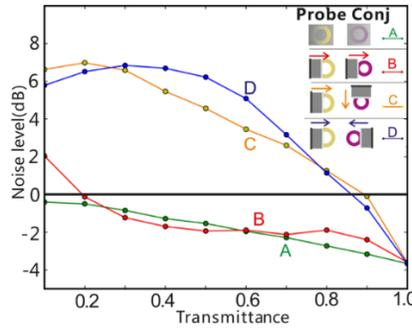
Fig. 3. The normalized intensity difference noise levels as a function of the transmittance as the two beams are attenuated equally. Probe: Probe; Conj: Conjugate. (A) The two beams are globally attenuated with a variable beamsplitter. The two beams are attenuated with razor blades cutting from (B) the same direction, (C) the perpendicular direction, and (D) the opposite direction.
