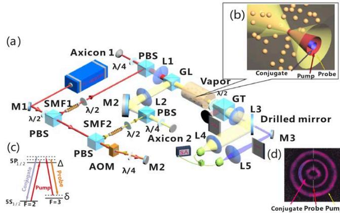
FIG. 1. The scheme and experimental layout for generating multi-spatial-mode quantum states of light via FWM process using conical probe and pump beams.
