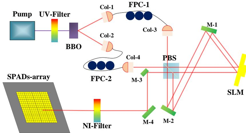
Fig 1. Experimental schematic. M ~ mirror. FPC ~ fiber polarization controller. Col ~ fiber collimator.
