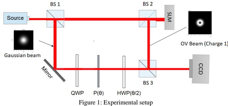
The azimuthal phase dependence of the vortex beam results in an off-center dark spot in the interference pattern, on superposition with the Gaussian beam. When the geometric phase is varied by changing the intermediate polarization states in one branch, the bright spot revolves around the common center of the superposed beams by an angle equivalent to the geometric phase shift ( $\phi_g$ ).
