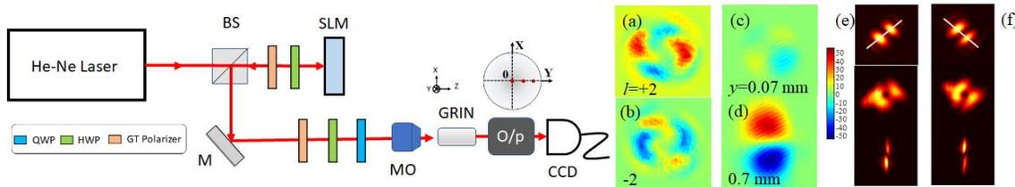
Fig. 1. Experimental setup and measurements of (a), (b) reciprocal spin-to-orbital angular momentum conversion; (c), (d) reciprocal spin-Hall effect and (e), (f) reciprocal orbital-Hall effect of light. Red and blue color in (a) – (d) correspond to right and left spin components in the beam.
